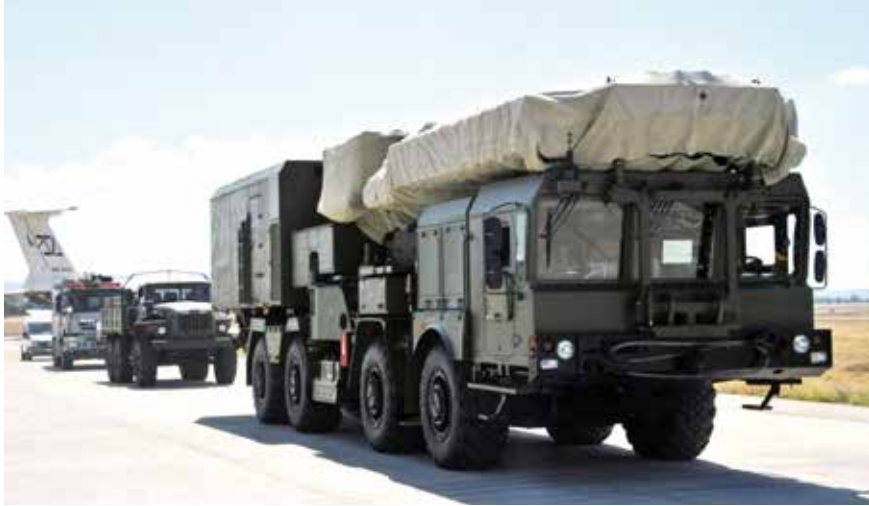
The 96L6E Surveillance and Tracking Radar of the Russian S-400 system being deployed in Turkey
